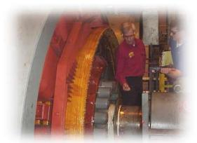
As a result, when Flanders built the new motors for the Logan mill, they made sure to include an Accumetrics Motor Monitor to constantly monitor the temperature of the armature. By continuously monitoring the internal temperature of the motors, the motors can run at a safe but full rating. Additionally, the mill operators can shut down the mill before a rise in temperature causes damage that would require an expensive and time-consuming rebuild.
